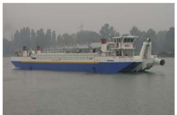
Self loading Dregder 60mt. Shipyard Costruzioni Navali Sarani - Italy
